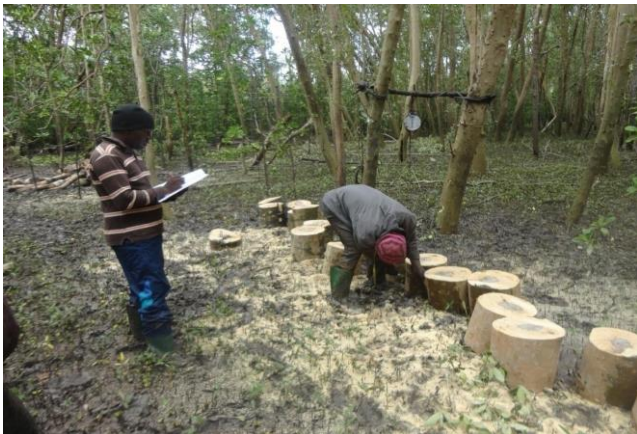
Figure 3. Recording diameters of billets before weighing in Rufiji River Delta, Tanzania (Photo: Lupembe 2013)
