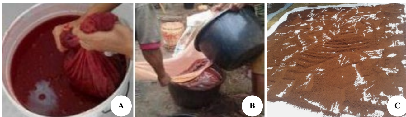
Figure 4. Wet extraction technique. A. Extraction using water media, B. Filtering process, C. Drying process under the sun
