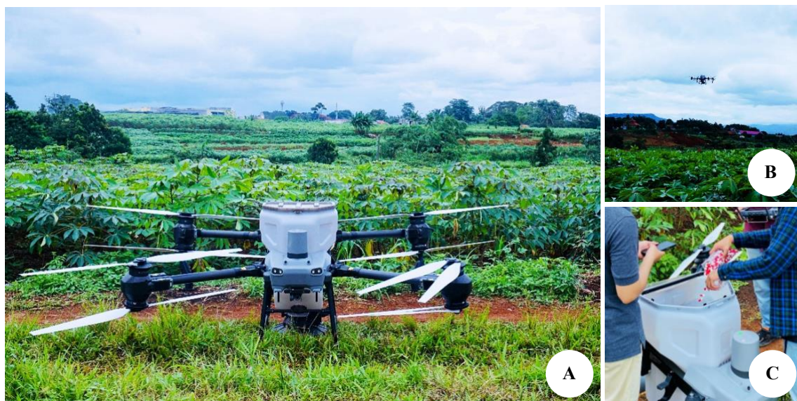
Figure 1. A. DJI Agras T50 Spreading System drone used for parasitoid capsule distribution. B. Drone-assisted release of parasitoid capsules in cassava fields. C. Insertion of parasitoid capsules into the drone tank
