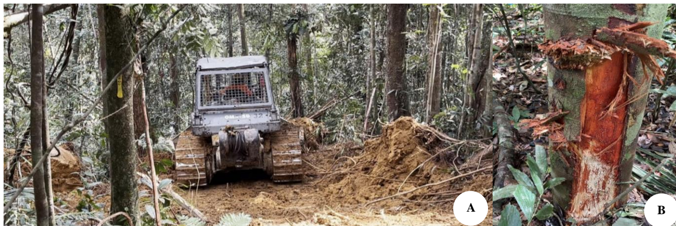
Figure 4. A. The process of creating skid road before tree felling; B. Stem wounds during skidding
