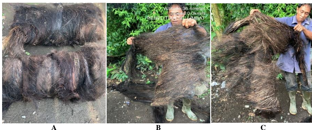
Figure 6. Black fiber. A. Ijuk roll, B. Small roll of ijuk , C. Big roll of ijuk
