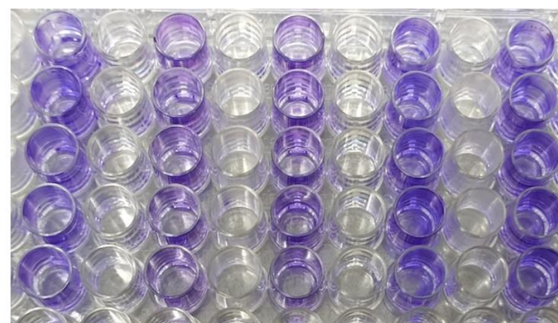
Figure 3. Biofilm inhibition after 72 hours' incubation in microtiter plate biofilm assay stained with 0.1% crystal violet
