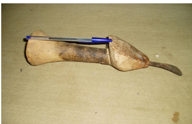
Figure 2. Mengaf is the traditional tool for tapping the Boswellia tree. Source. Ali et al. (2009)
