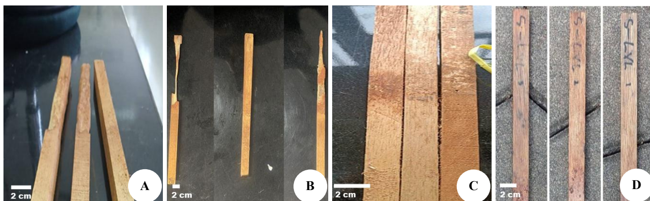
Figure 2. Visual appearance of wood samples after a 3-month soil burial test. A. Solid Jabon (JS) and B. Jabon LVL (JL) show severe degradation characterized by deep penetration, longitudinal hollowing, and substantial loss of structural integrity. In contrast, C. Solid Sengon (SS) and D. Sengon LVL (SL) exhibit only minor surface erosion with largely intact cross-sections, indicating superior resistance to biological deterioration. All samples had identical dimensions (2×2×40 cm) and were exposed to the same soil moisture and microbial conditions
