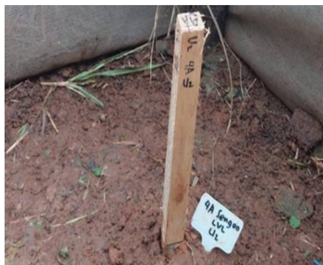
Figure 1. Graveyard (field-stake) test setup for evaluating natural wood durability according to ASTM D1758-06. Individual wood specimens (2×2×40 cm) were buried vertically in soil to a depth of 20-30 cm, leaving the upper portion exposed
