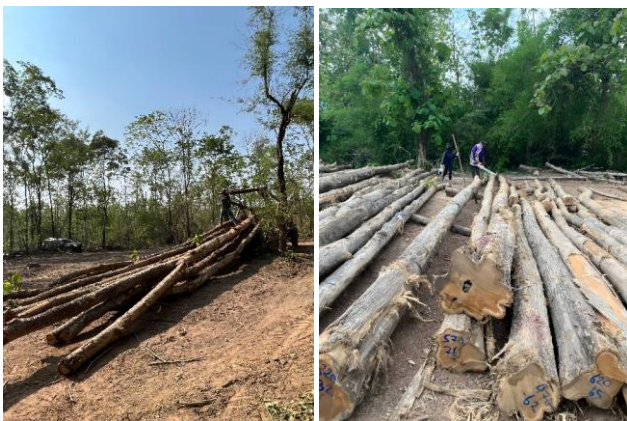
Figure 4. Skidding of tree-length logs by truck to the log yard for chainsaw bucking
