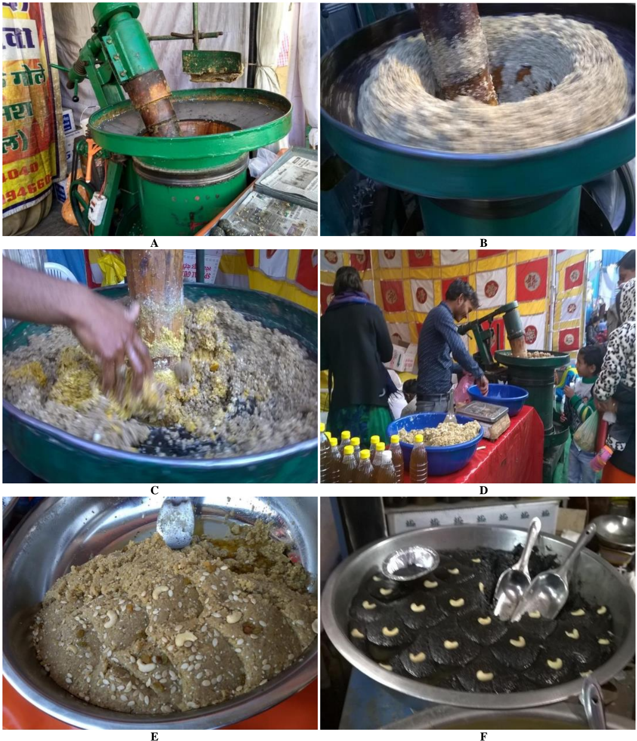
Figure 1. A. Electric ghani , B. Milling sesame seed in Ghani , C. Mixing of jaggery, D. Selling of jagal in the fair, E. Jagal prepared from white sesame seeds, F. Jagal prepared from black sesame seeds
